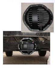
Aftermarket **rear differential covers** are not only aesthetical pleasing, but they serve a very functional purpose; better cooling. With a larger oil capacity than stock, in this case 25% more, and cooling fins, aftermarket diff covers help **reduce heat** in the rear diff, especially under stressful driving conditions, such as those encountered when off-road. The added thickness also adds strength to the differential housing.
